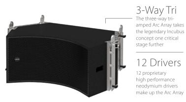
An all-new four-point rigging system with a range of tilt angles from 0° to 10° in five discrete increments makes rigging Arc Array a safe and simple experience for system techs. Housed in a heavily braced 15mm birch plywood enclosure with road proven TourCoat polyurea finish, Arc Array is designed for efficient trucking and handling. Two Neutrik speakON<sup>™</sup> NL8s are provided for driver connections.
